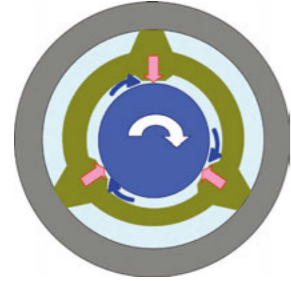
砥石軸受 マッケンゼンタイプ非接触油動圧軸受 Grinding wheel bearing Mackensen type non-contact hydraulic bearing.
